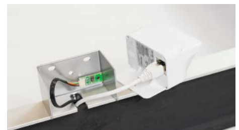
LED Occupancy Sensor & Anti-sweat Sensor Connected
